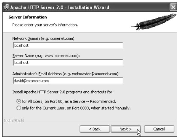
Figure 2-3. Filling out the Server Information dialog box during installation of Apache
